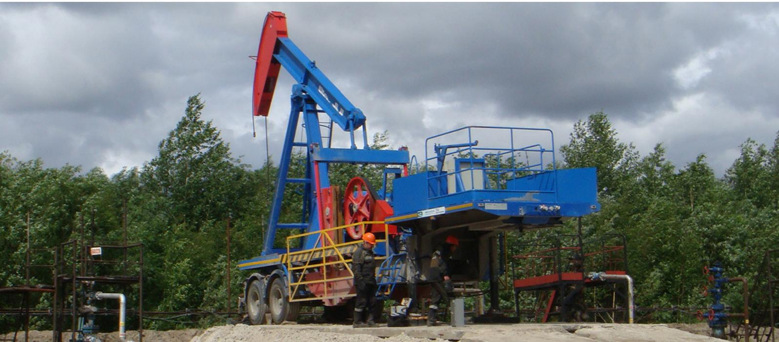
1. Mobile Pumping Unit driven by an electric motor (hereinafter called as Mobile Unit) is intended for individual mechanical drive of sucker rod pumps for test short-term service of reactivated or new wells to determine their productivity and other characteristics. It allows proper selection of a stationary pumping unit size for well operation.
